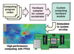
High-performance computing with a hardware structure tailored to target application
