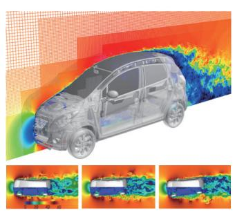
Simulation of coupled vehicle aerodynamics and 6DoF-motion utilyzing CUBE
