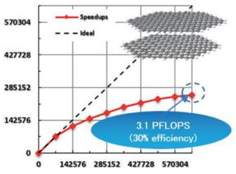
Parallel efficiency of the electron-correlation calculation with NTChem on the K computer
