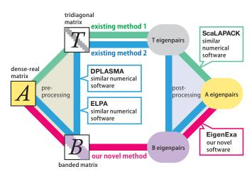
Schematic view of a new scheme
