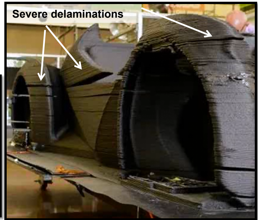
Delaminated product after production
